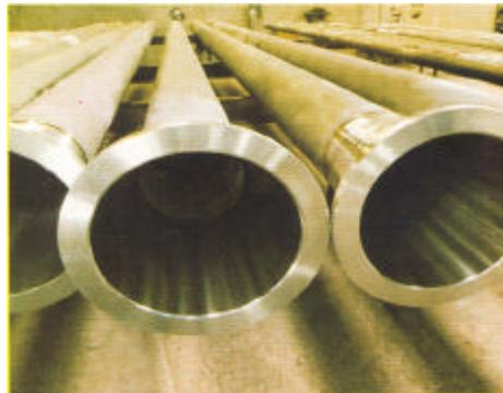
Some of the Reformer Tubes Supplied to a Direct Reduction Steel Plant.
